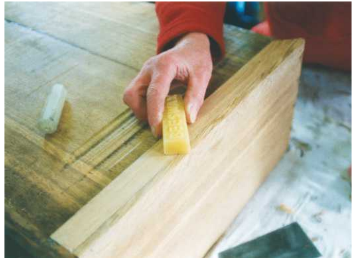
▲ Pic.5 ...wax the new runners so that they glide from the outset
